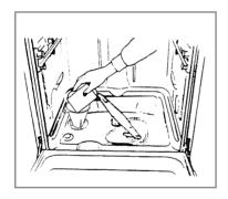
The salt container must be filled when the "low salt" indicator light (located on the control panel) comes on.
